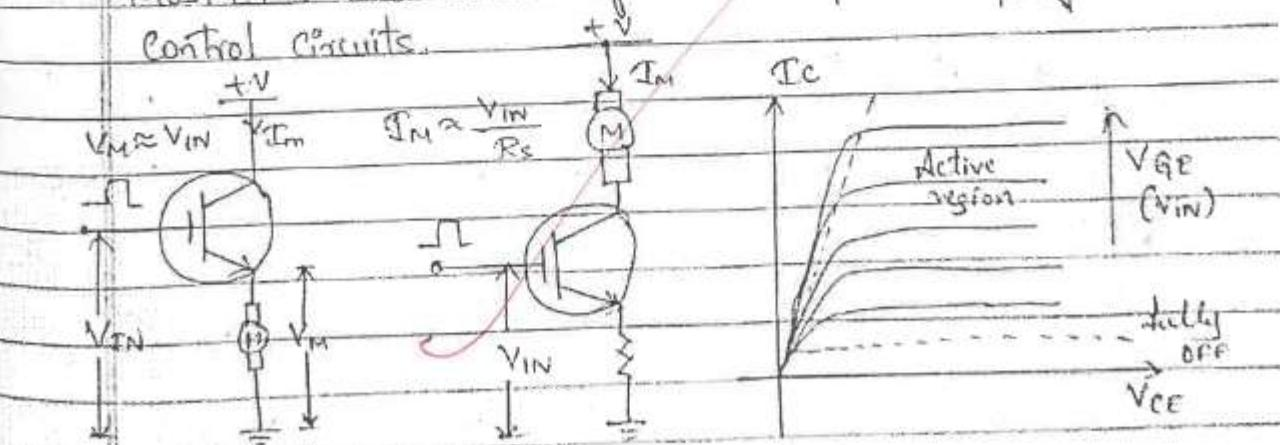
\* Since the IGBT is a voltage controlled device, it only requires a small voltage on the Gate to maintain conduction through the device unlike BJT's which require
