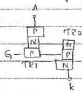
\* The two transistor equivalent circuit shows that the collector current of the NPN Transistor TR2 feeds directly into the base of the PNP Transistor TR1, while the collector current of TR1 feeds into the base of TR2.
