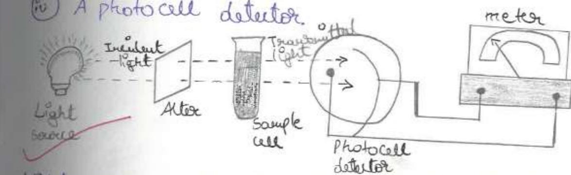
Light from a tungsten lamp is allowed to fall on the soln taken in the sample cell after passing through the filter. First, a blank soln is taken in the sample cell & placed in the path of the light beam. Its absorbance is adjusted to zero (or transmittance to 100) on the meter. Next the analyte soln is placed in the path of the light beam & the quantity of light absorbed is measured at its absorbance (or transmittance).
