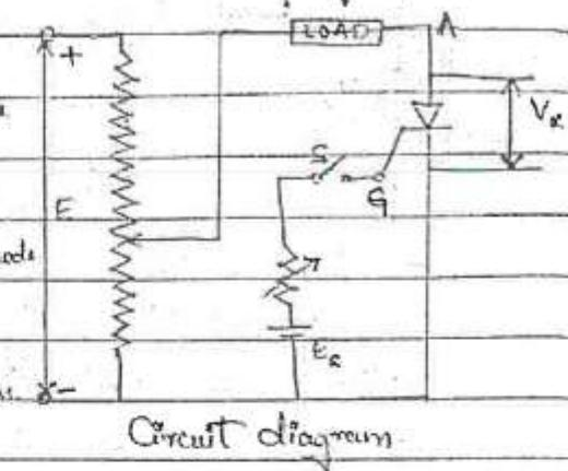
\* Initially for the reverse blocking mode of the thyristors, the cathode is made positive with respect to anode by supplying voltage  $E$  and the gate to cathode supply voltage  $E_g$  is detached initially by keeping switch 'S' open.
