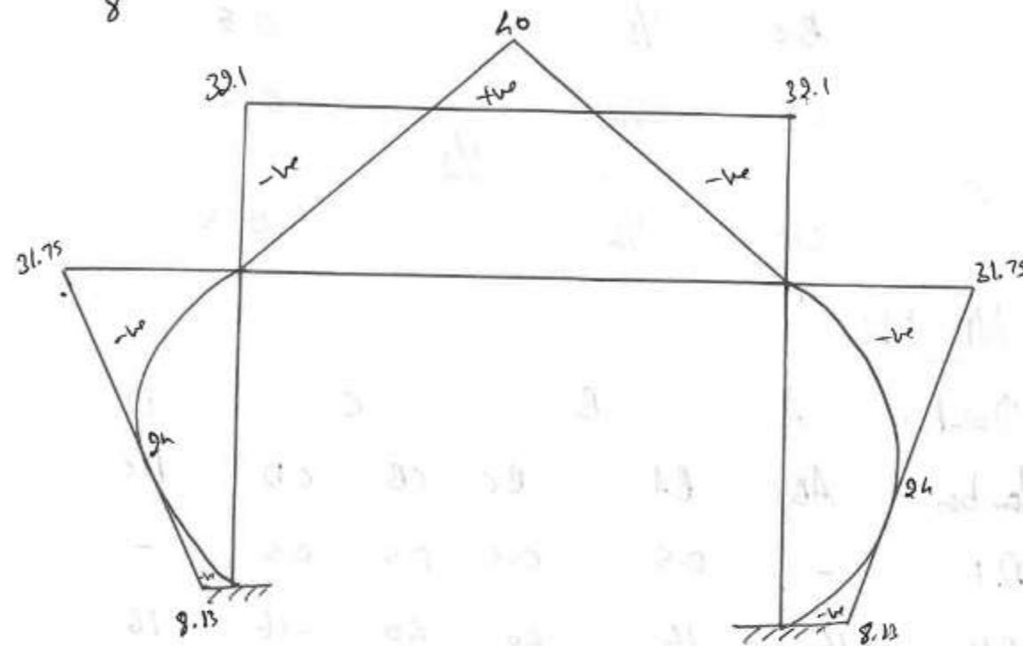
3. Analyse the beam shown in fig. 3 using Kanish method
