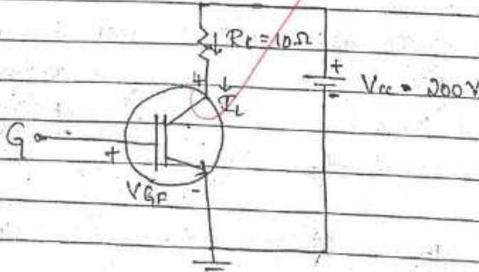
Soln:  $T_{on} = 3 \mu\text{sec}$ ,  $T_{off} = 1.2 \mu\text{sec}$ ,  $D = 0.7$ ,  $V_{ce(sat)} = 2 \text{ V}$ ,  $f_s = 1 \text{ kHz}$
