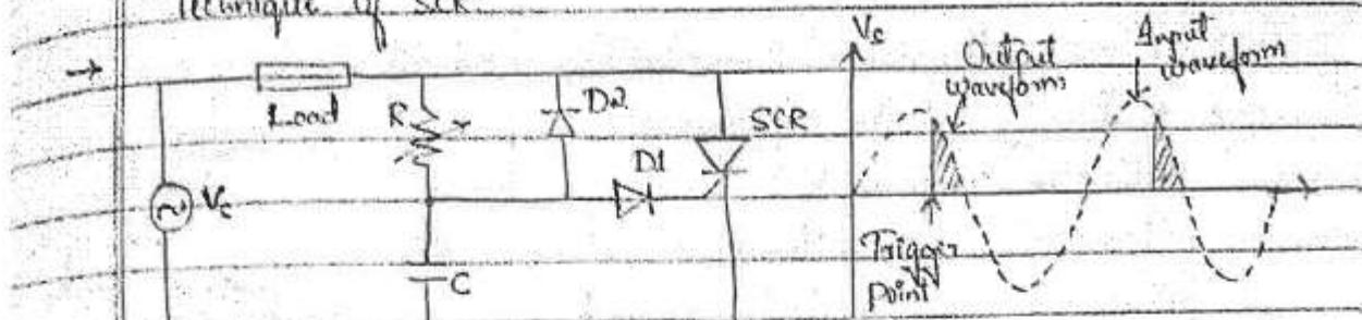
\* The limitation of resistance fixing circuit can be overcome by the RC Triggering Circuit which provides the firing angle control from 0 to 180 degrees. By changing the phase and amplitude of the gate current, a large variation of firing angle is obtained using this circuit.
