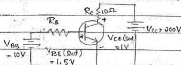
Soln:  $B = 8 \text{ to } 10, \text{ ODF} = 5, R_c = 10\Omega, V_{CE(sat)} = 1V, V_{BE(sat)} = 1.5V, V_{CC} = 200V, V_{BB} = 10V$
