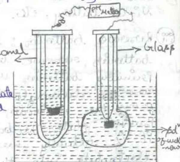
The emf of the cell so formed is determined potentiometrically.
