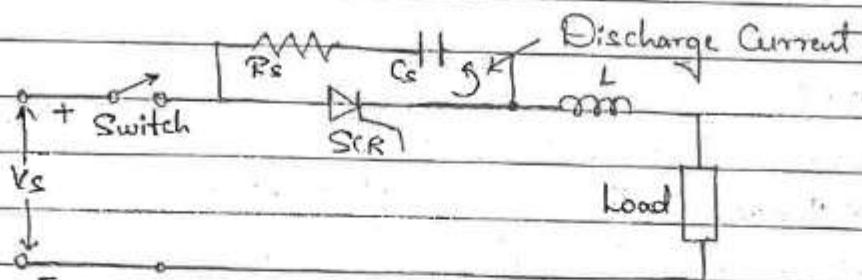
\* The protection against high voltage reverse recovery transient &  $dv/dt$  is achieved by using an RC snubber circuit.
