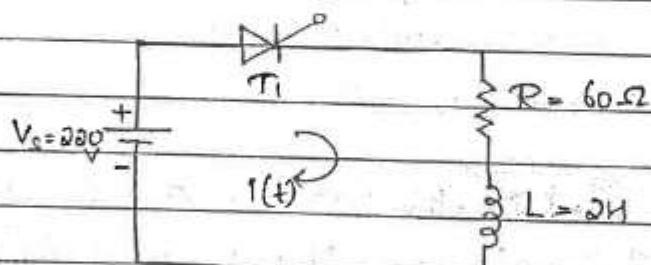
$$\text{Pulse width} = 10 \mu\text{sec}, I_L = 36 \text{ mA}, R = 60 \Omega, L = 2 \text{ H}$$
