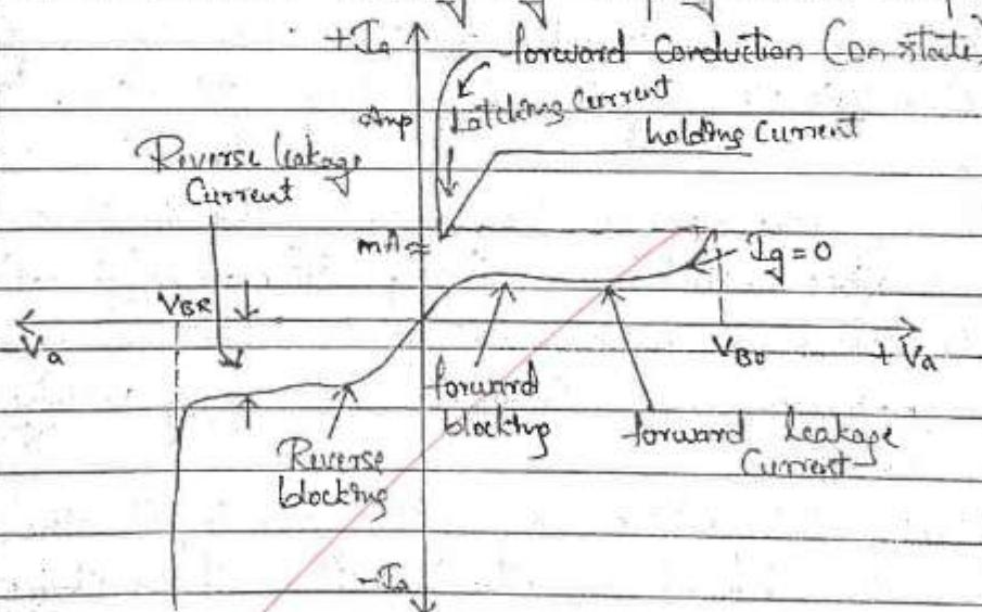
\* When the anode to cathode forward voltage is increased, with gate circuit open, the reverse junction  $J_2$  will have an avalanche breakdown at forward break over voltage  $V_{BO}$  leading to thyristor turn on.
