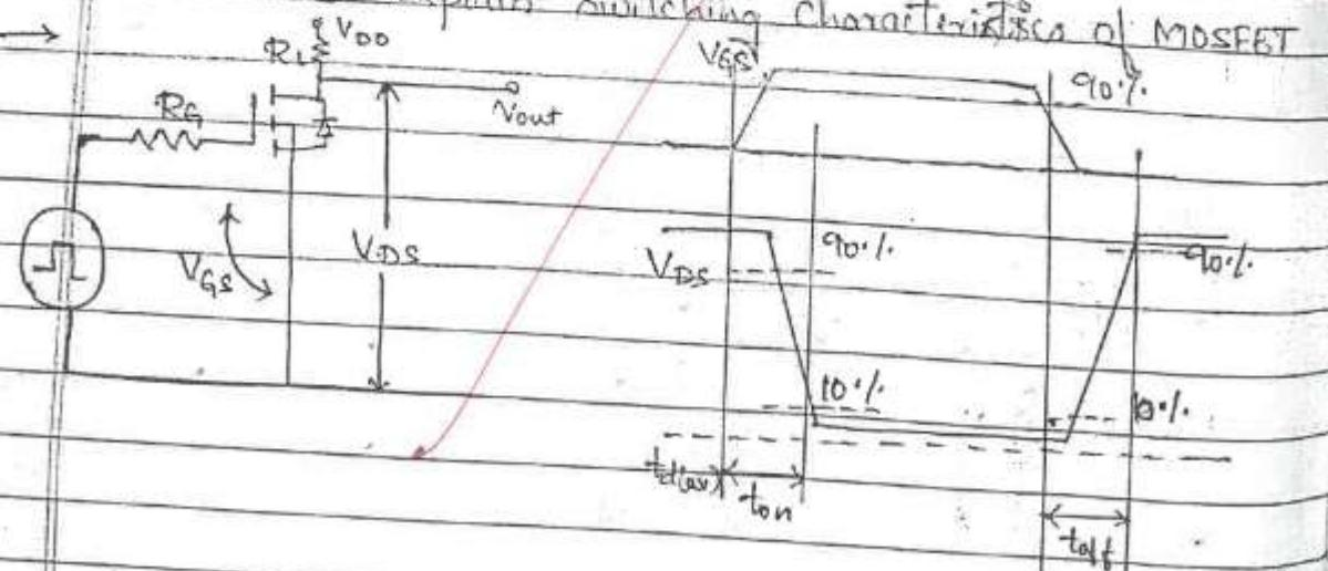
\* Since power MOSFET's are majority-carrier devices, they are faster and capable of switching at higher frequencies than bipolar transistors.
