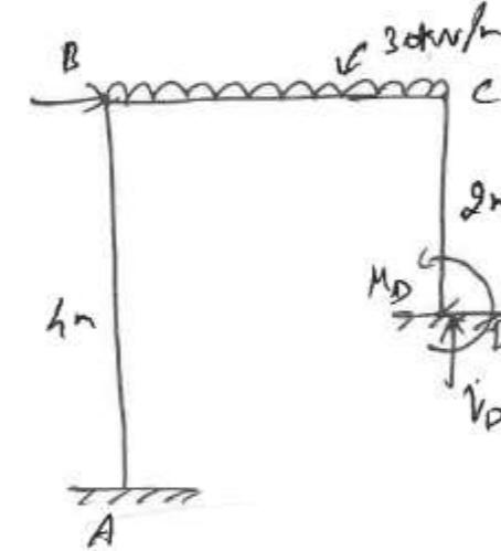
$$M_B = M_D + V_D \times h - H_D \times 2 - 30 \times h \times \frac{h}{2}$$
